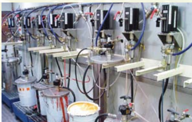
2-ball piston pumps 4:1 ratio, used in a painting process manufacturing
