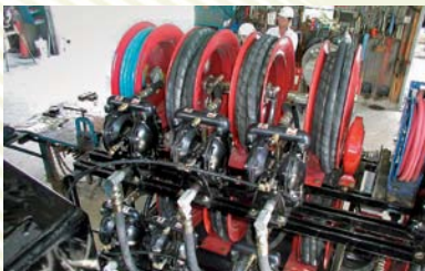
UL approved fuel pump 1" size, used assembled on skid dedicated in the aviation to fill and unload kerosene
